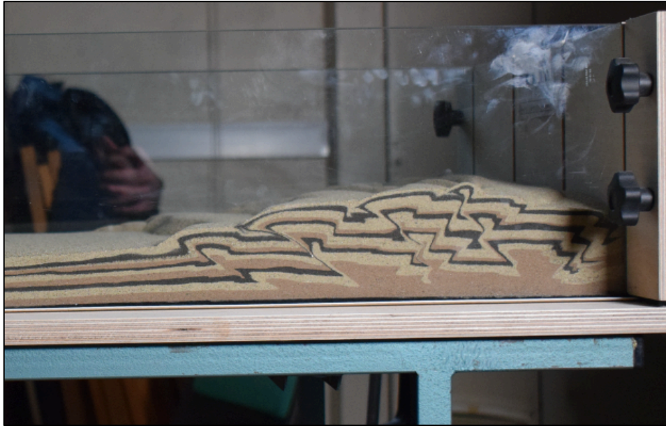
Figure 2.6 - Sandbox experiment for a previous course representing plate convergence. The model shows the internal structures of an accretionary wedge. Folds and thrusts verge in opposite directions meaning that relying simply on vergence is not enough to determine the tectonic processes.
