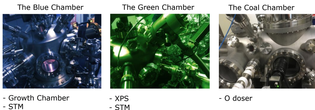
Figure 5.1: The UHV chambers used in the project, named the Blue, Green, and Coal chamber. Reprinted from [116].
