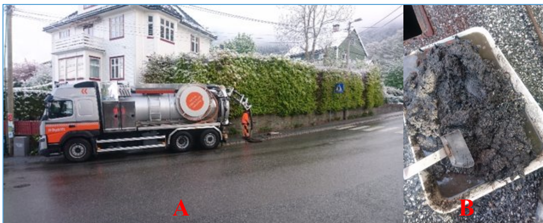
Figure 7: A) The vehicle removing overwater from sand traps. B) Sediment collected with a stainless-steel sampling spoon. Photo: Einar Bye-Ingebrigtsen, NORCE
