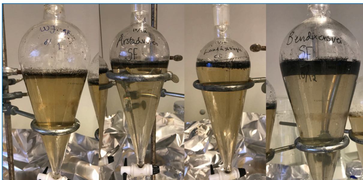
Figure 12: A selection of samples in glass separation funnels during the second density separation with \text{ZnCl}_2 , showing abundant microplastic and TWP. From left to right: Suburban4TR, Suburban1TR, Suburban2TR, Suburban3TR.
