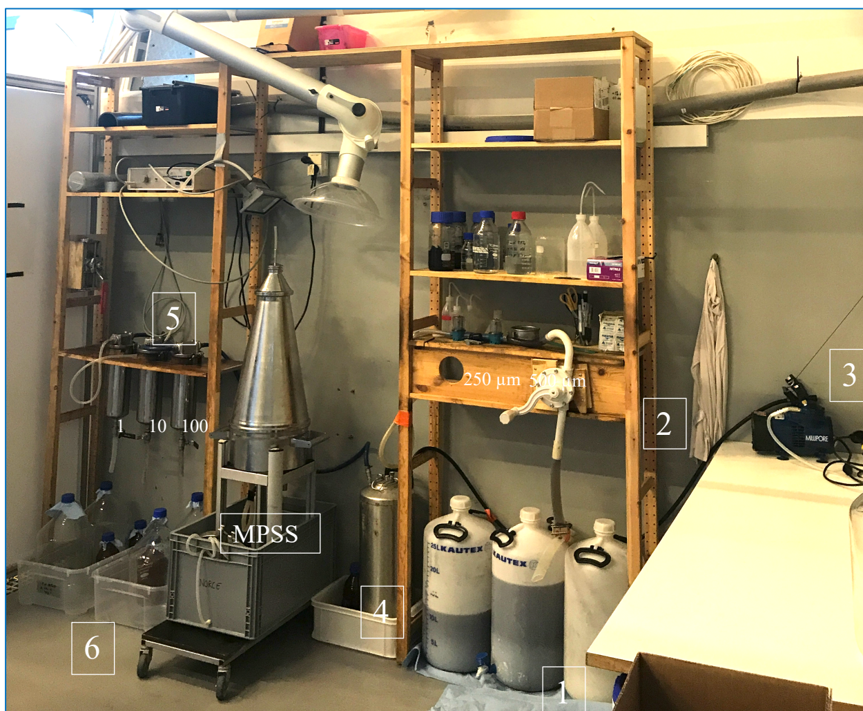
Figure 9: The filtration process for reusing \text{ZnCl}_2 . 1 – Sedimentation of \text{ZnCl}_2 after MPSS analysis. 2 – Manual pump for unclean \text{ZnCl}_2 filtered through two filters of 500\ \mu\text{m} and 250\ \mu\text{m} , respectively. 3 – Compressor (Chemical Duty Pump Model WP6111560, Millipore, USA). 4 – Pressure container for 250\ \mu\text{m} filtered \text{ZnCl}_2 , attached to pressure hose for compressed air from 3. 5 – Stainless steel cylinder filter containers, from right to left: 100\ \mu\text{m} stainless-steel filter (Rolf Körner GmbH), 10\ \mu\text{m} glass fiber filter (GF/C filter, Hytrex Catrige), 1\ \mu\text{m} GF/C filter (Hytrex Catrige). These filters were clean or exchanged when the filtration process considerably slowed down. 6 – Clean \text{ZnCl}_2 ( < 1\ \mu\text{m} particle size) qualified for sample processing, stored in precleaned glass bottles.
