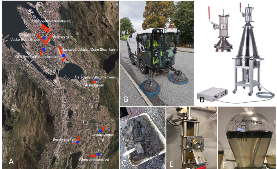
Pictures show the sample locations (red lines = SS, blue dots = ST) (A), the vehicles assisting in the sampling of SS (B), a sediment sample from ST prior to analysis (C), the MPSS (Hydro-Bios) used for MP extraction (D) a sample during the second density separation, showing abundant MP and TWP particles (F)
