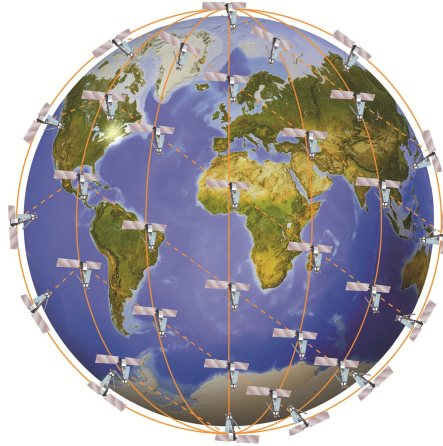
Figure 3.6: A schematic view of the distribution of satellites in the Iridium constellation. Image courtesy of ESA [2012] .
