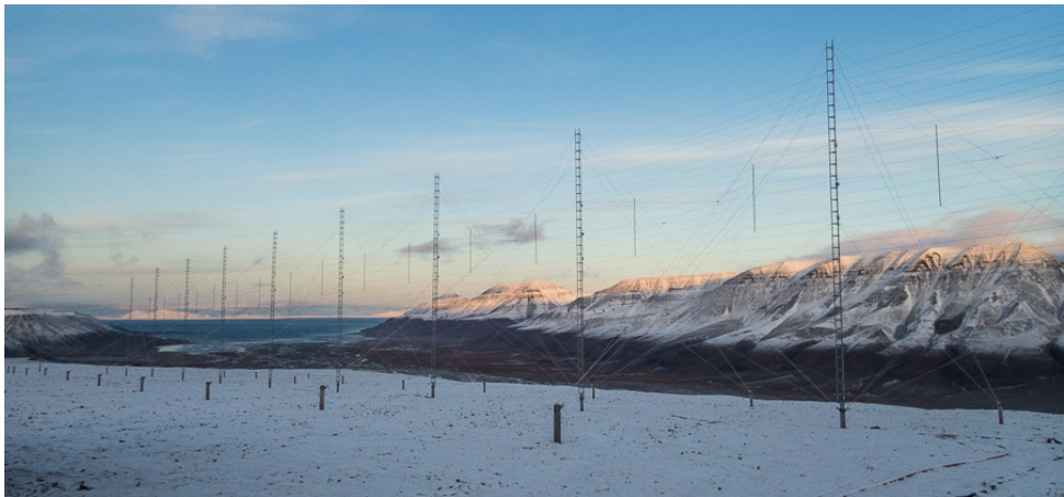
Figure 3.2: Image of a section of the main antenna array of the SuperDARN Longyearbyen radar. Image courtesy of Mikko Syrjäsuo (UNIS) [2017] .
