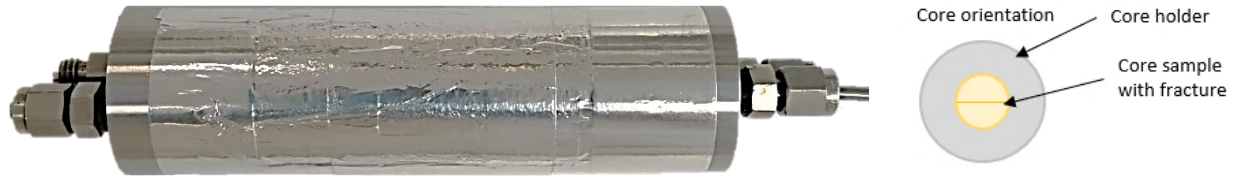
Figure 3.7 – On left-hand side, the core sample and end pieces wrapped in aluminum foil for preventing CO 2 migration. On the right-hand side, the core sample orientation.
