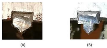
Figure 3.4 – (A) Sharp edges used to split core samples in experiment L1, L2 and L3. (B) New modified sharp edges used to split core sample L4 and L5.
