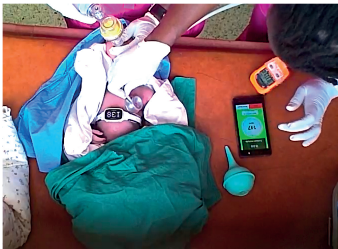
Figure 2 Low-end user using NeoTap to record heart rate (heart rate shown 147) and dry-electrode electrocardiography (heart rate shown 138). Picture used with written permission from the parents.
