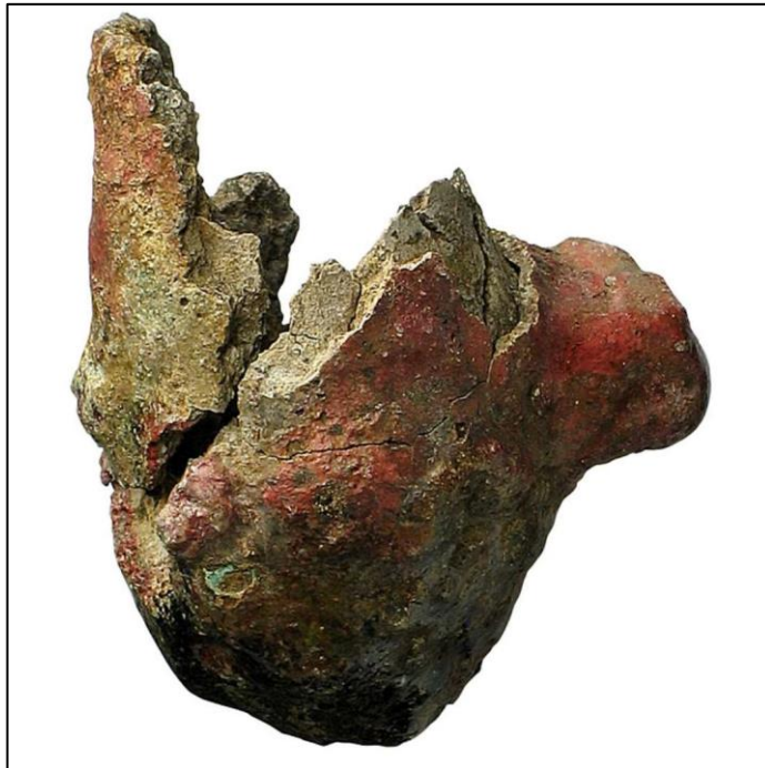
Fig. 5.2: Type 2 crucible from Ribe with a lug in the middle (ASR 9x311, left) and a type 2 crucible fragment from Birka with the lug along the rim (SHM85975, above) (Images: SHM and SJM).
