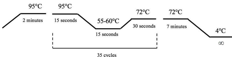
**Figure 11** The thermoprofile used during Polymerase Chain Reaction in a thermocycling machine. Stage 1: 2 minutes of denaturation at 95°C. Stage 2: 35 cycles of denaturation at 95°C for 15 seconds, annealing at 55-60°C for 15 seconds and elongation at 72°C for 30 seconds. Stage 3: 7 minutes of final extension at 72°C.
