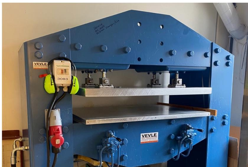
**Figure 8** Image of the hydraulic press used to press fish filets in vacuum bags.
