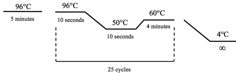
**Figure 12** The thermoprofile used during the sequencing-reaction. Stage 1: 5 minutes of denaturation at 95°C. Stage 2: 25 cycles of denaturation at 95°C for 10 seconds, annealing at 50°C for 10 seconds and elongation at 60°C for 4 minutes.
