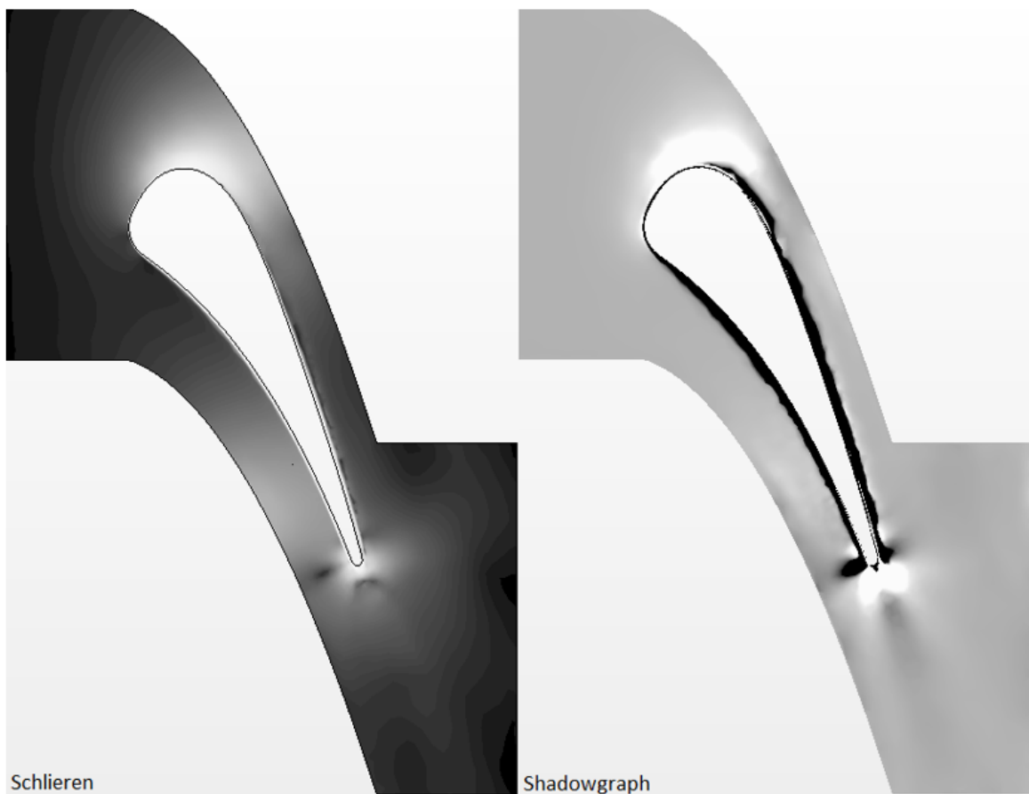
Fig. 5.3 Numerical Schlieren and shadowgraph image of the flow over the C3X vane.
