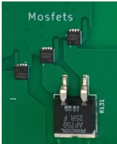
(a) MOSFETs which control the charging, discharging, and load of the supercapacitor
