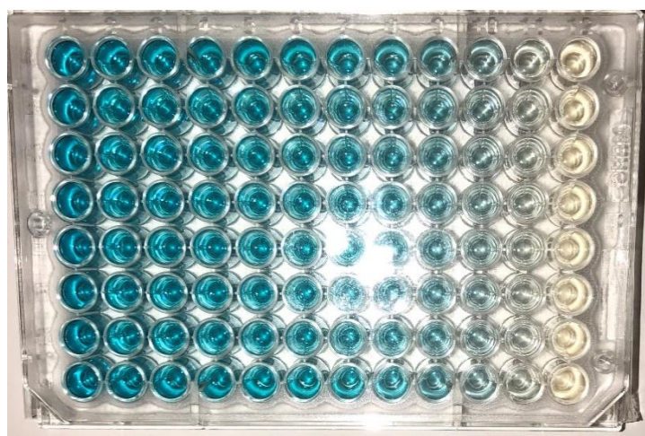
Figure 2.5: 96-well microtiter plate filled with serial dilutions of copper sulphate pentahydrate, starting with the highest concentration in the left column.
