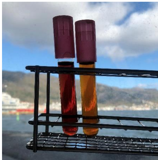
Figure 2.4 After incubation, tubes containing enterococci would change colour from dark red (left) to ochre yellow (right).
