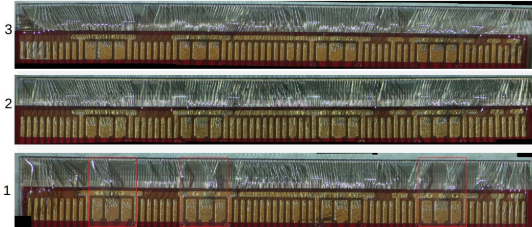
Figure 6.20: A picture of the wirebonds on the module chips. This was done using a Olympus microscope with Canon EOS MK II camera.
