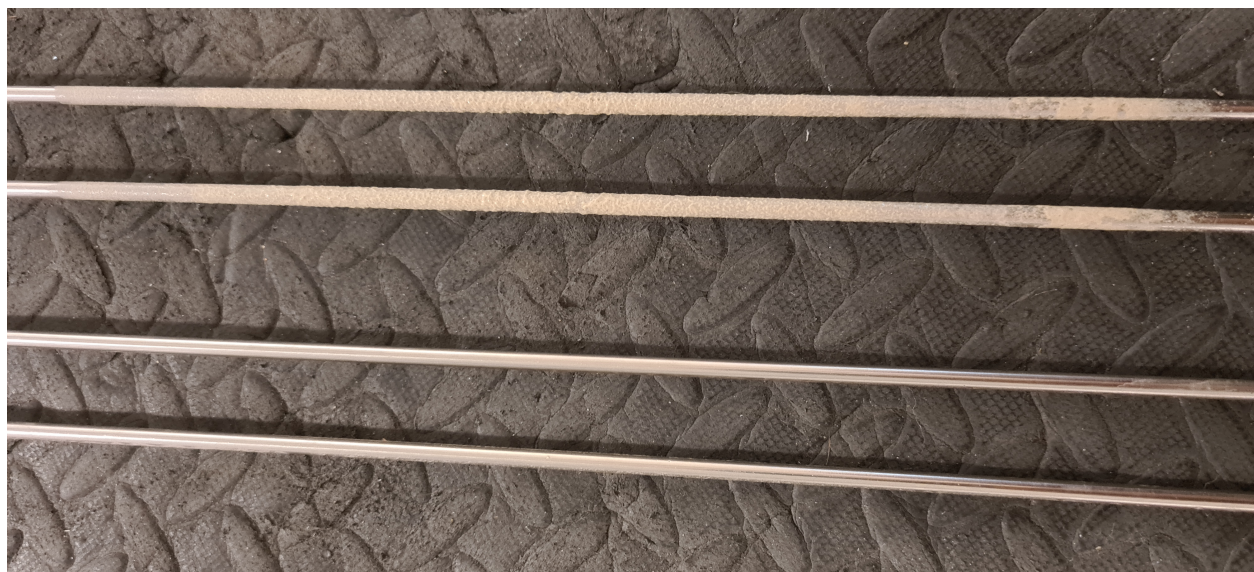
Figure 11: Two different wave gauges with the upper wave gauge showing how the seeding particles have gathered on the probes near the water surface.
