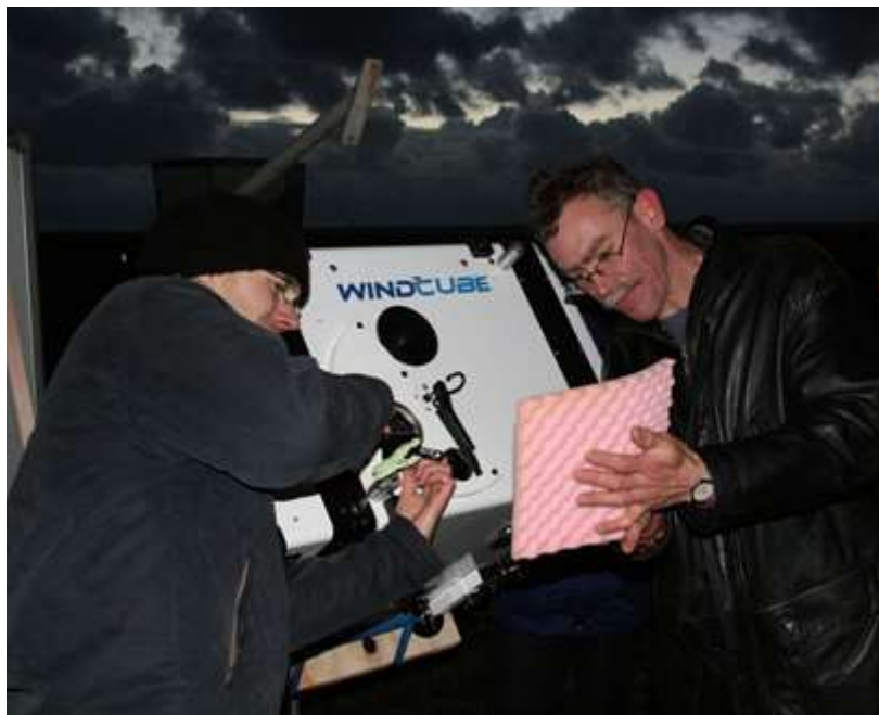
Fig. 3: The first DTU Wind Energy Musketeer experiment using three staring wind cubes. Jean-Pierre Cariou and Remy Parmentier from Leosphere aligning an alignment laser at a cold December evening at Høvsøre, western Jutland, Denmark.
