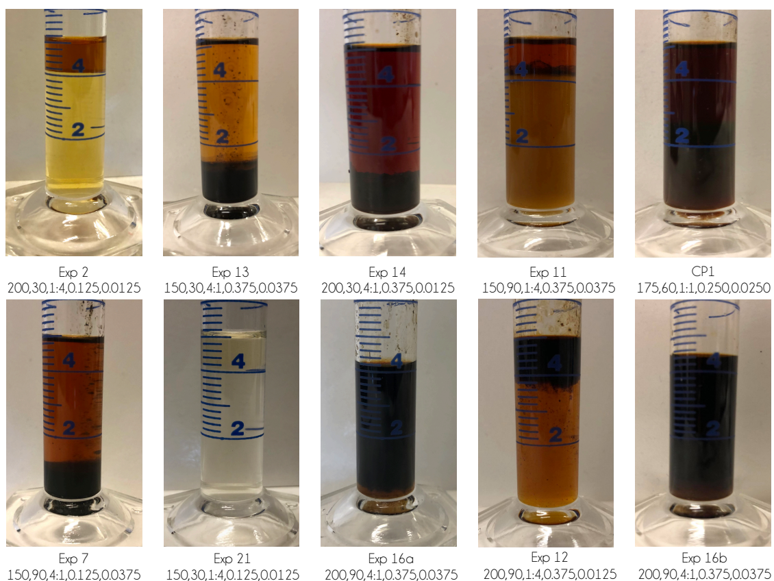
Figure 5-18: Product solutions from FFD1. Reaction conditions for each experiment is listed under each picture ( T(^{\circ}\text{C}), t(\text{min}), \text{org}: \text{aq}(\text{vol}/\text{vol}), \text{substrate}(\text{g}), \text{catalyst}(\text{g}) ).
