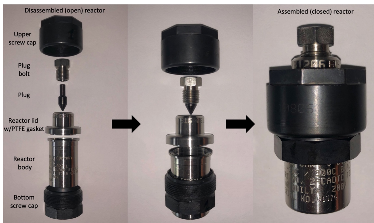
Scheme K-6: Pictures of a Series 4700, 316 Stainless steel batch Parr reactor (22mL) with a polyphenylene lining. The picture to the left shows the different reactor parts when the reactor is disassembled.
