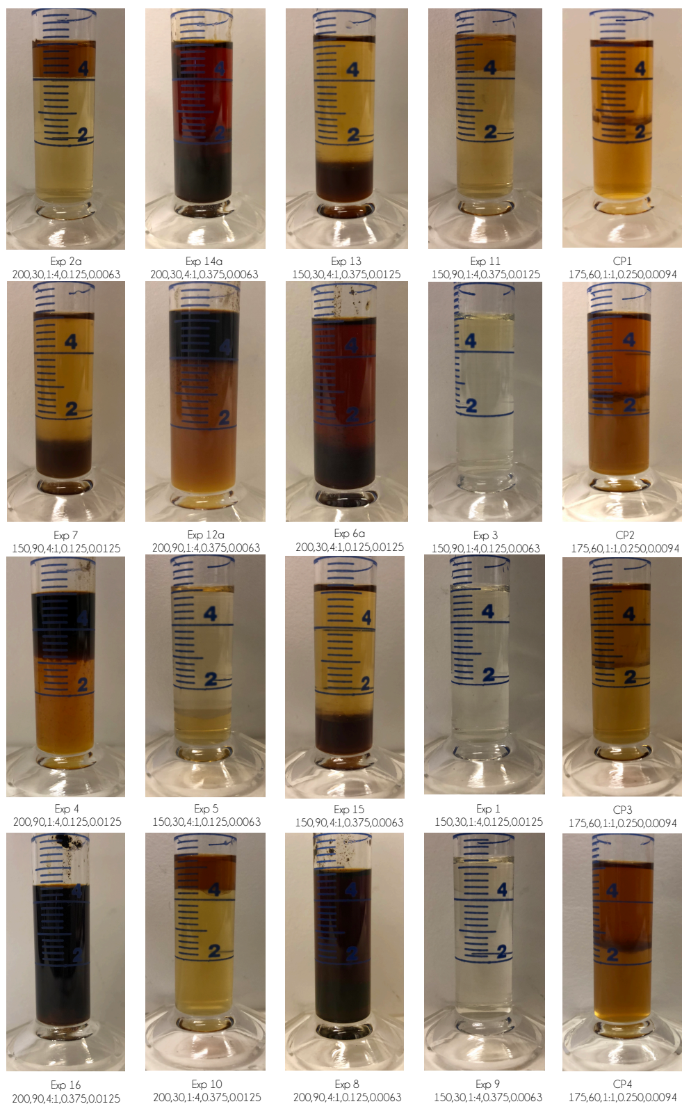
Figure 5-21: Product solutions from FFD2. Reaction conditions used for each experiment is listed under each picture ( T(^{\circ}\text{C}), t(\text{min}), \text{Org:aq}(\text{vol/vol}), \text{substrate}(\text{g}), \text{catalyst}(\text{g}) ).
