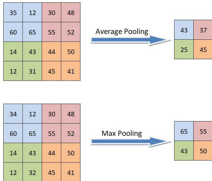
Figure 14: Outputs of a 2x2 average pooling and a 2x2 max pooling layer (modified from Yani et al., 2019).
