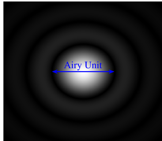
Figure 2.6: The Airy disk simulated from the squared Sombbrero function using MATLAB. The Airy Unit is drawn in with the blue arrow.
