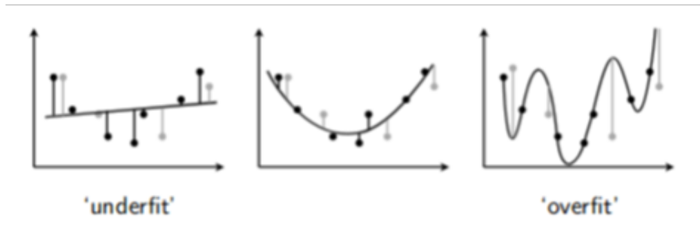
Figure 2.1: Illustration of an underfitted (left), a well-fitted (middle) and an overfitted (right) model to the data [84].
