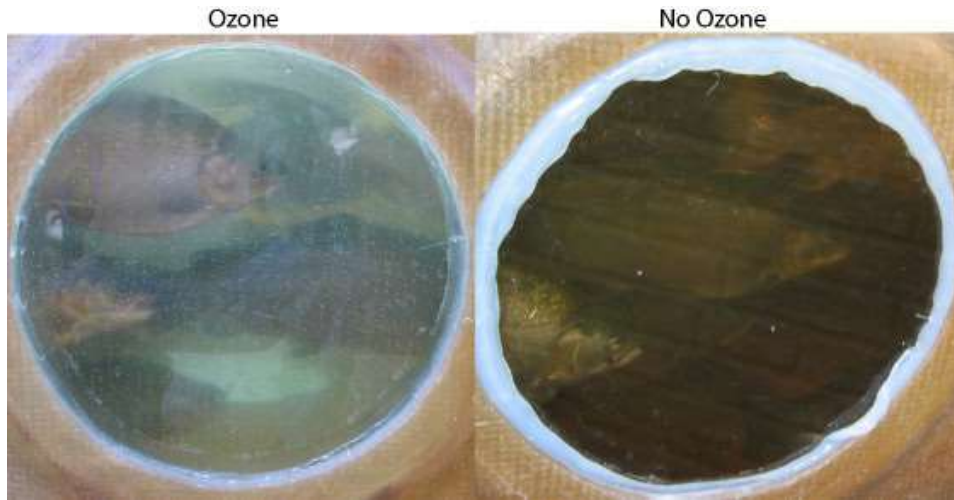
Fig. 4. Visual water quality differences observed through an observation portal for WRAS operated with and without ozone at low water exchange.
