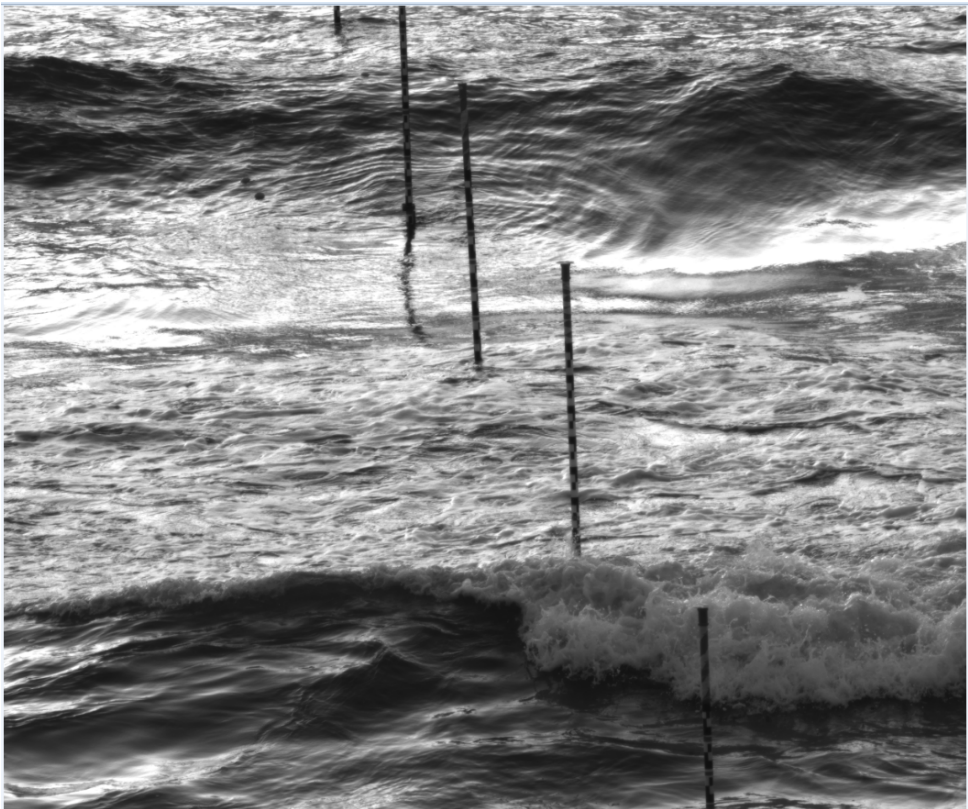
Figure 3.2: This is a single photo captured by the north camera (Camera 2) placed to the right on top of the ridge behind the beach. The five outermost poles can be seen together with three floating oranges. Two of the oranges are located to the left of pole 2, while one orange is located on top of the wave between pole 1 and pole 2.
