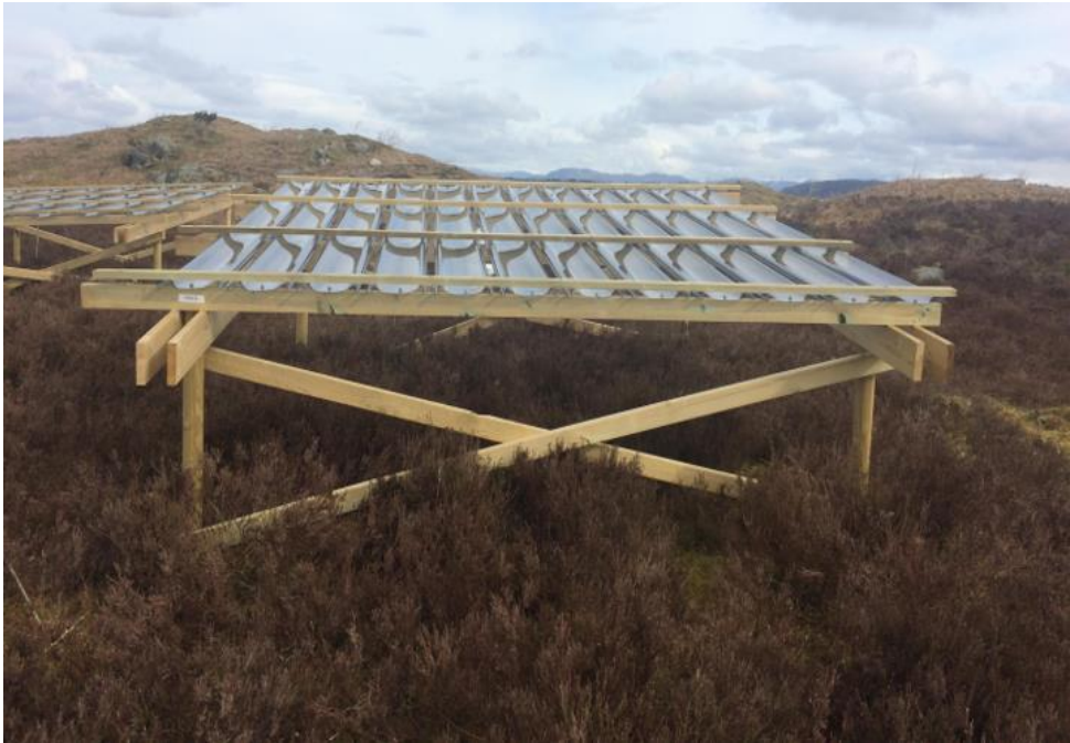
Figure 11: Photo of a rainout shelter with 90% roof cover, representing the extreme drought treatment. The shelter shown in the photo is installed on an intermediate successional phase plot in the south. Calluna dominates the vegetation and appears brown in the photo which was taken in spring. Nevertheless, these Calluna stands still have green shoots supporting livestock through winter. A moderate (60% roof cover) drought treatment plot is visible to the far left in the background. Photo: Siri V. Haugum.
