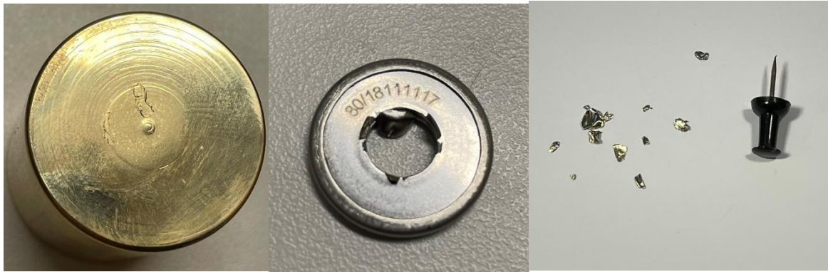
Figure 5-25 Grooves in OOC caused by impacts from debris (left). An open rupture disc (middle). Collected debris from all experiments. Thumbtack for size reference (right)
