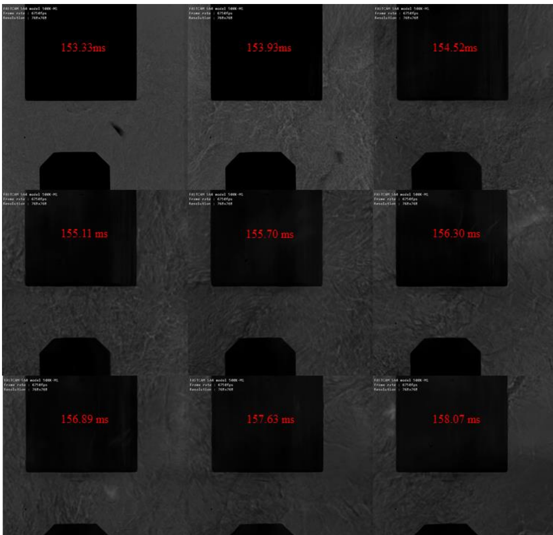
Figure 5-18 Timelapse for explosion development in a typical ignited test. Example shown is test 78.
