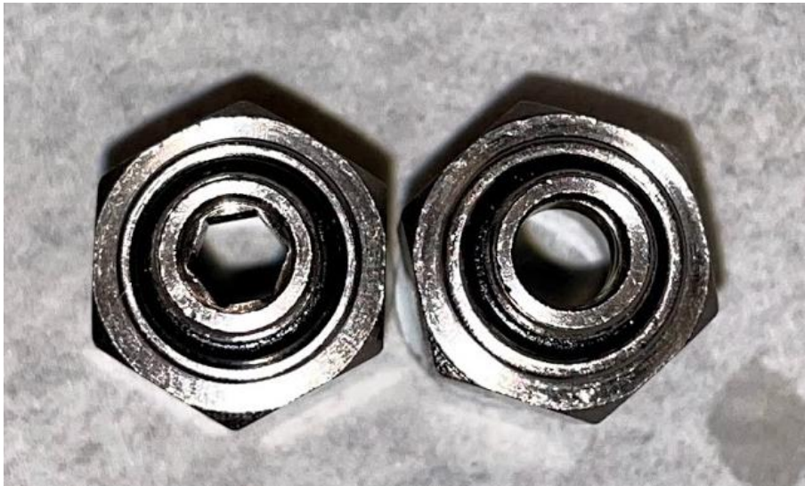
Figure appendix 11 The difference between an original G1/8" fitting for 10 mm hose and the modified version used for this application that was drilled with 5.8 mm
