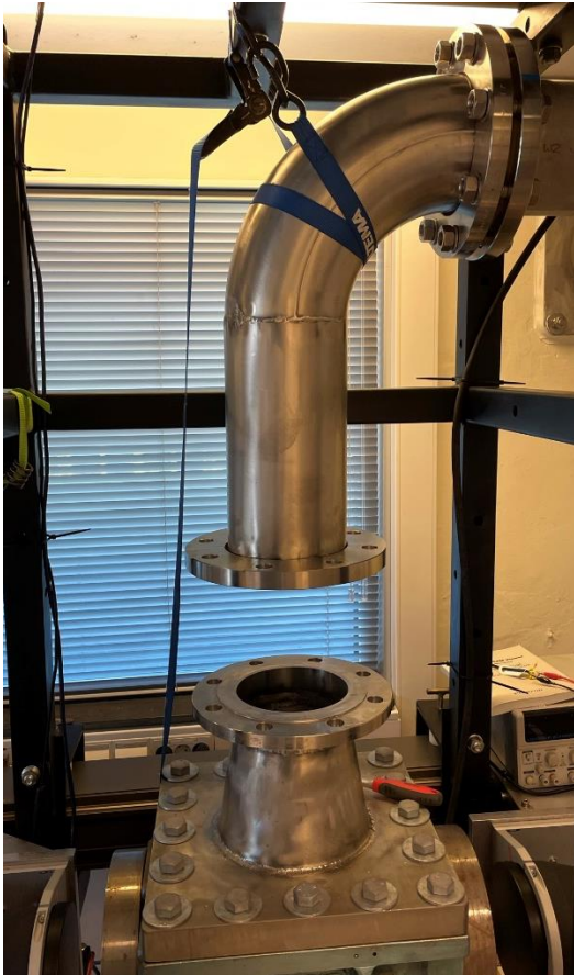
Figure 4-9: The lid of the 20-litre explosion vessel and the blowdown pipe, with the axial expansion joint removed.
