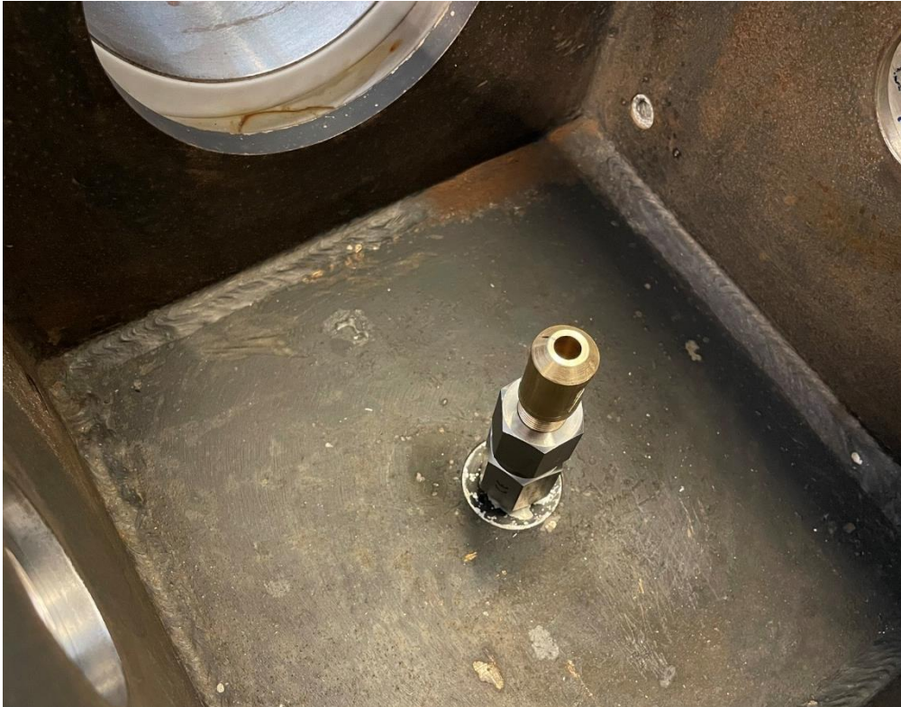
Figure 4-3: Rupture disc assembly installed in the explosion chamber (ID at nozzle exit = 8 mm).
