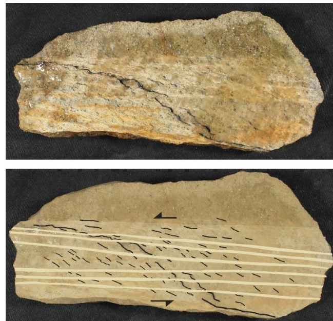
Figure 5.16: Hand sample of sample W5. Coal is sheared and rotated by deformation bands.
