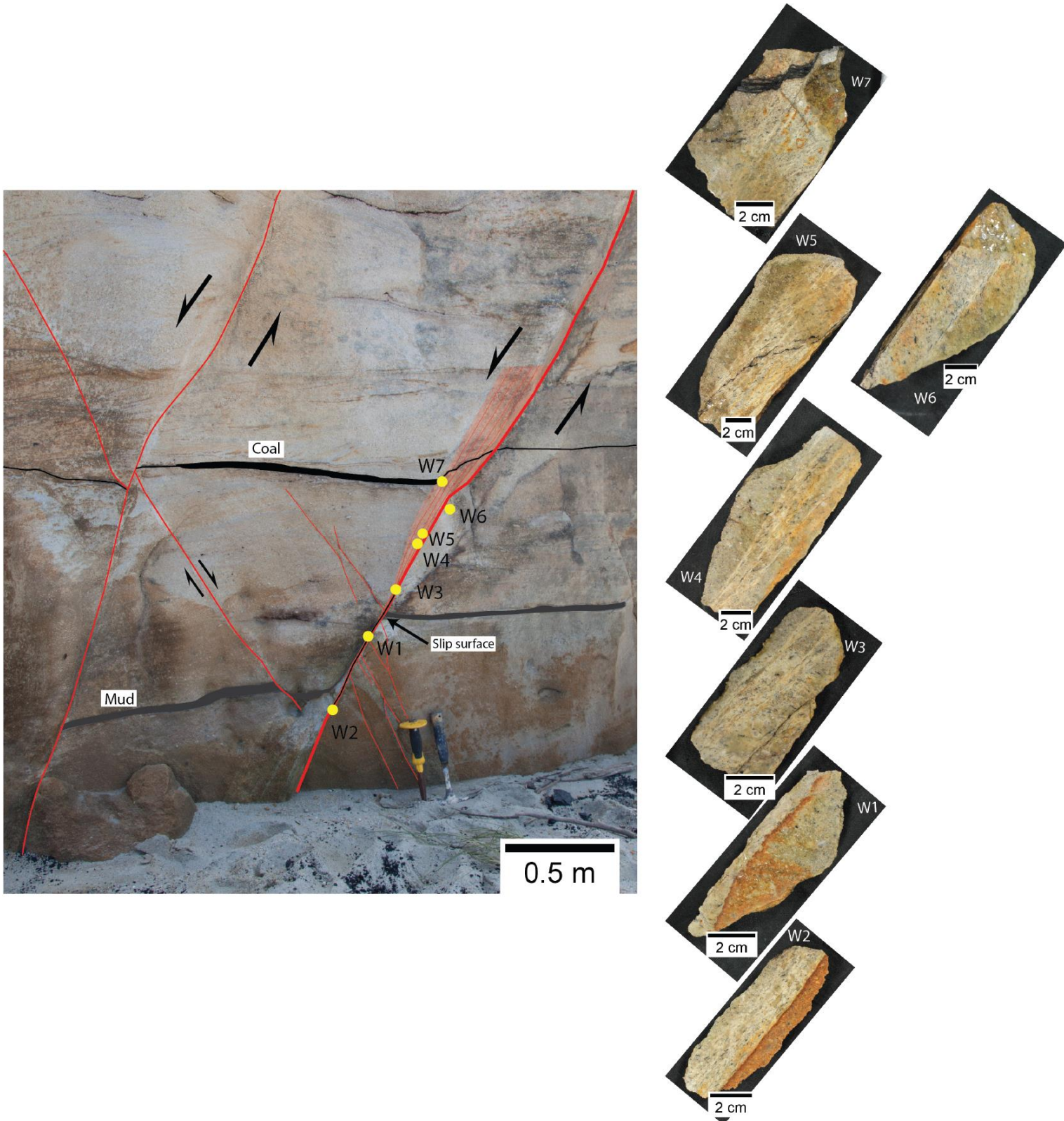
Figure 5.3: Picture of the studied location of sample set 1 and from where the samples were collected along the band. The red lines are deformation bands, and the cluster of interest is highlighted as a red zone. Black lines show the coal and mud layers that have been displaced. Photographs of each hand sample collected is included. The deformation bands in the hand samples are visible as slightly lighter colored bands.
