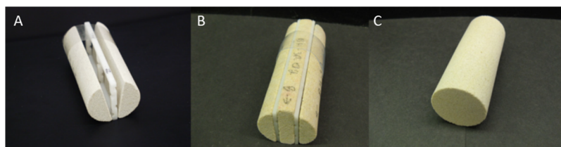
Figure 1. Core plug design of single fracture (A), double fracture (B), and unfractured (C) experiments. A POM spacer was placed in the fractures to maintain a constant fracture aperture during experiments. Reproduced from Birkedal et al. 22
