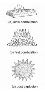
**Figure 1.** Illustration of the increase of the combustion rate of a given mass of combustible solid with increasing sub-division. From Eckhoff [1–3]. Copyright (2019), with permission from Elsevier.
