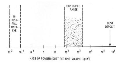
**Figure 2.** The range of explosible dust concentrations in air at normal temperature and atmospheric pressure for a typical natural organic dust (maize starch). A comparison with typical range of maximum permissible dust concentrations in the context of industrial hygiene, and a typical density of deposits of natural organic dusts. From Eckhoff [1–3]. Copyright (2019), with permission from Elsevier.
