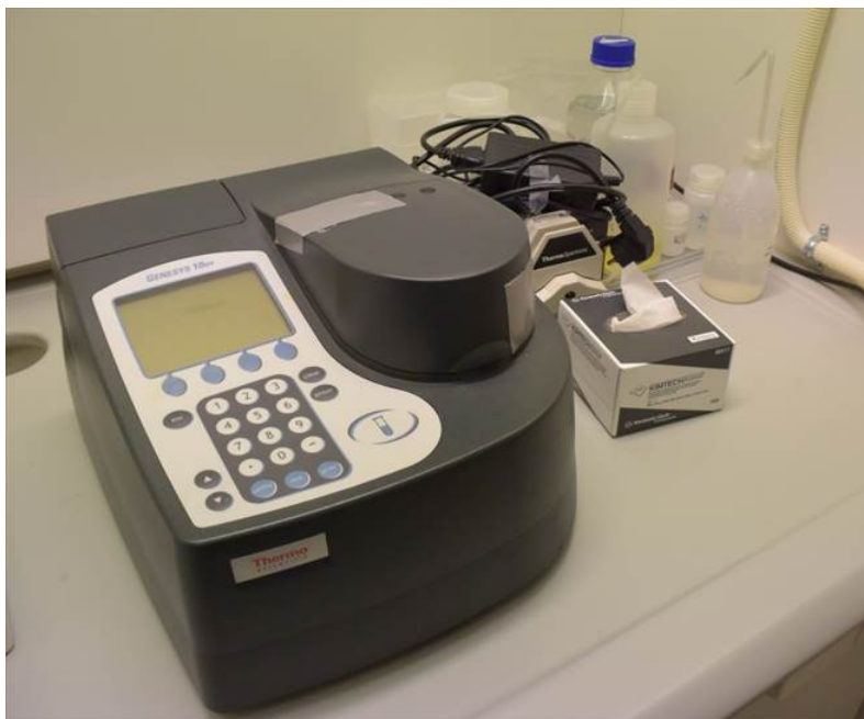
Figure 4.4: The UV-VIS spectrophotometer used for the iron concentration measurements. Picture taken by Desiree Lisette Roerdink.
