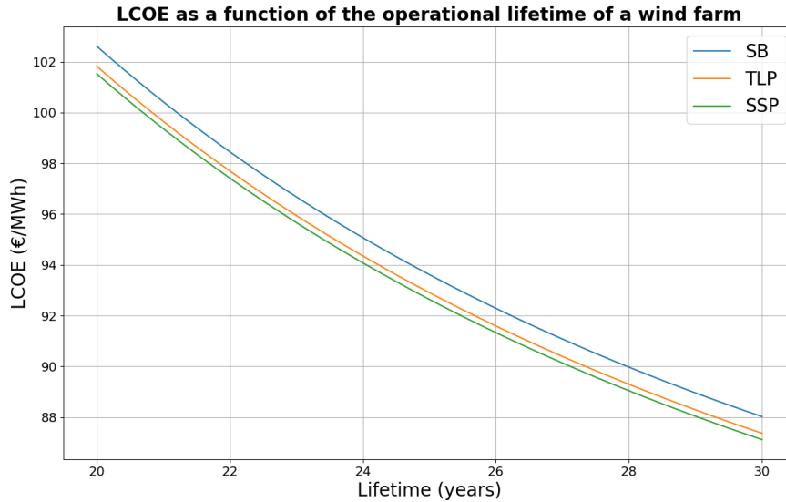
Figure 5.7: The graph shows LCOE of a wind farm as a function of the wind farm’s operational lifetime. All other wind farm parameters than the lifetime used in the results in this figure can be found in table 5.1, which gives an overview of the reference wind farm. LCOE (€/MWh) is shown on the y-axis, while the lifetime (years) is shown on the x-axis. The graph displays the LCOE of three different wind farms, using the SB (blue line), the TLP (orange line), and the SSP (green line) as the floating platform.
