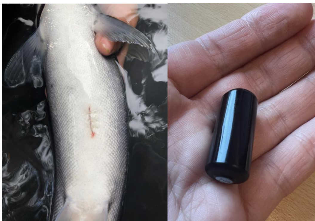
Appendix 2. Picture of a tagged sea trout (left) and the acoustic transmitter (right).
