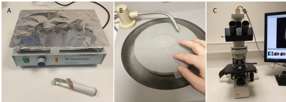
Figure 4: Process of otoliths for microstructure analysis. Otoliths glued on marked microscope slides with help from a hotplate and crystal bond (A), grinding machine with sandpaper (P2500) (B), and microscope with camera attached to a computer for visualization and for photographing microstructure (C).
