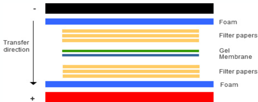
Figure 5. Schematic picture of western blot wet transfer sandwich (ref: https://www.sinobiological.com/category/wb-wet-transfer )
