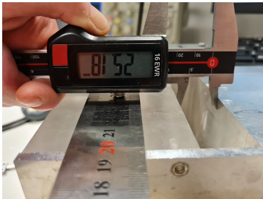
Figure 3.11: A picture illustrating the limitation on measurements due to the knife-edge's length using the digital caliper MarCal 16EWR.
