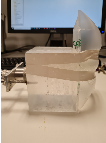
Figure 3.12: Picture of the measurement setup used to measure the sound velocity in the Plexiglas as a function of temperature. A plastic bag filled with air is secured with tape on the back of the Plexiglas, and a transducer is clamped onto the front. The setup is immersed into the water bath
