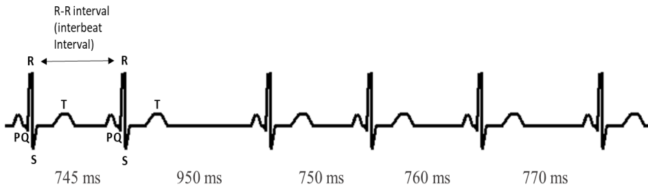
Figure 1.1. Illustration of an ECG recording. The deflections of the ECG are named P, Q, R, S and T, respectively. The distance between two R-deflections is called an R-R-interval, and make up an IBI. Varying IBIs, due to activity of the ANS, results in HRV.
