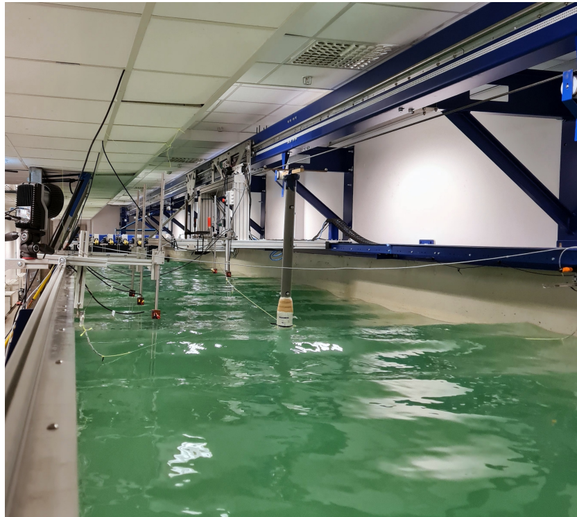
Figure 3.4: The complete experimental setup with the spar-buoy in MarinLab, a hydrodynamic research facility at HVLs campus in Bergen.
