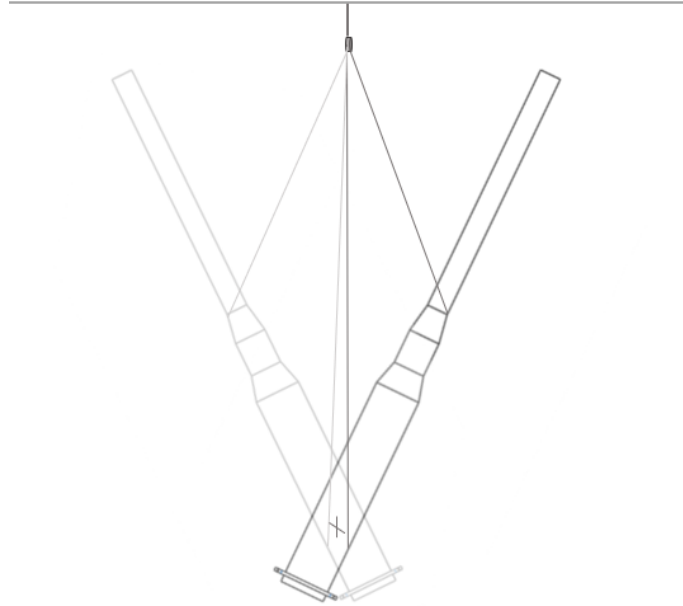
Figure 3.2: Sketch of the Bifilar suspension method used to estimate the location of the spar buoy's center of gravity without the top mass included.
