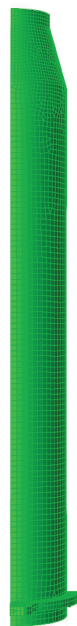
Figure 4.3: 1/4 panel model used in OrcaWave for diffraction/radiation analysis with a mesh element-size of 1 meter.
