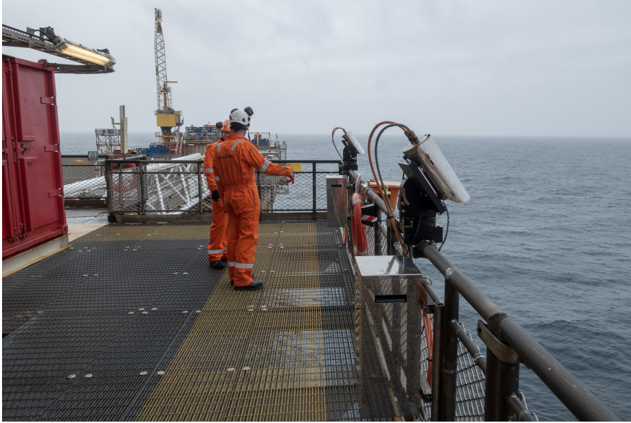
Figure 3.4: The Ekofisk stereo camera system in February 2019. Note that the stereo camera viewing angles in this photograph are steeper than in the current (post-August 2019) configuration used in this work. The white frame in the background belongs to the footbridge connecting the K and B platforms which houses the LASAR instrument. Photo by the author.
