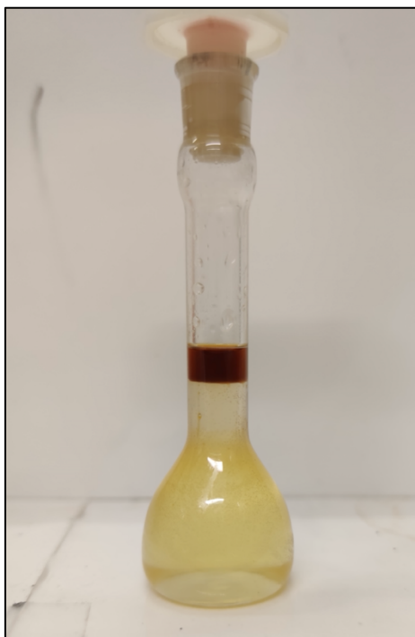
Figure E-3. Picture of the 10mL volumetric flask the organic phase was extracted with water in, after refrigeration.
