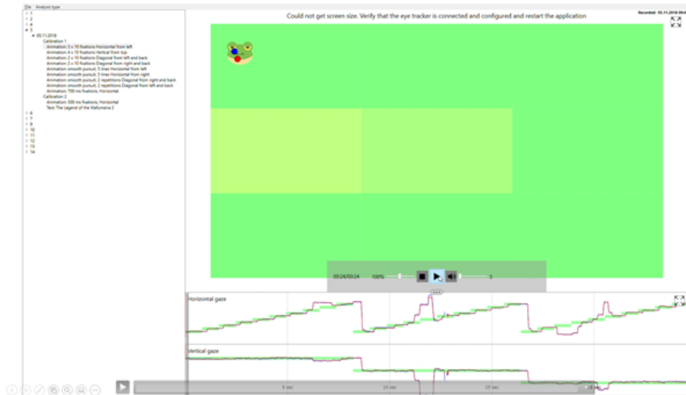
Figure 2.10: The user interface of C&Look during playback of a test. The stimulus object seen as a frog and recording data at the bottom. The position of the eyes can be seen as the two circles on the stimulus object. (Watanabe & Eide, 2017)
