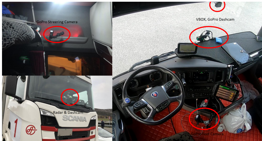
Figure 2.1: The sensor setup for one truck. Image credit: M.Eitrheim, M.Log et al. Edited by: F.Vindenes
