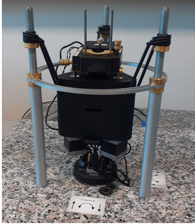
Figure 4.14: Picture of the AFM instrument "Eddy" from Anfatec, used in this thesis
