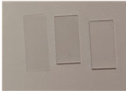
Figure 4.2: Picture of the different sample surfaces used for measurements in this thesis. Smooth silica (left) with thickness 0.1 mm, width 5.0 mm and length 12.0 mm. Smooth sapphire (middle) and rough sapphire (right) with thickness 0.5 mm, width 5.0 mm and length 10 mm.
