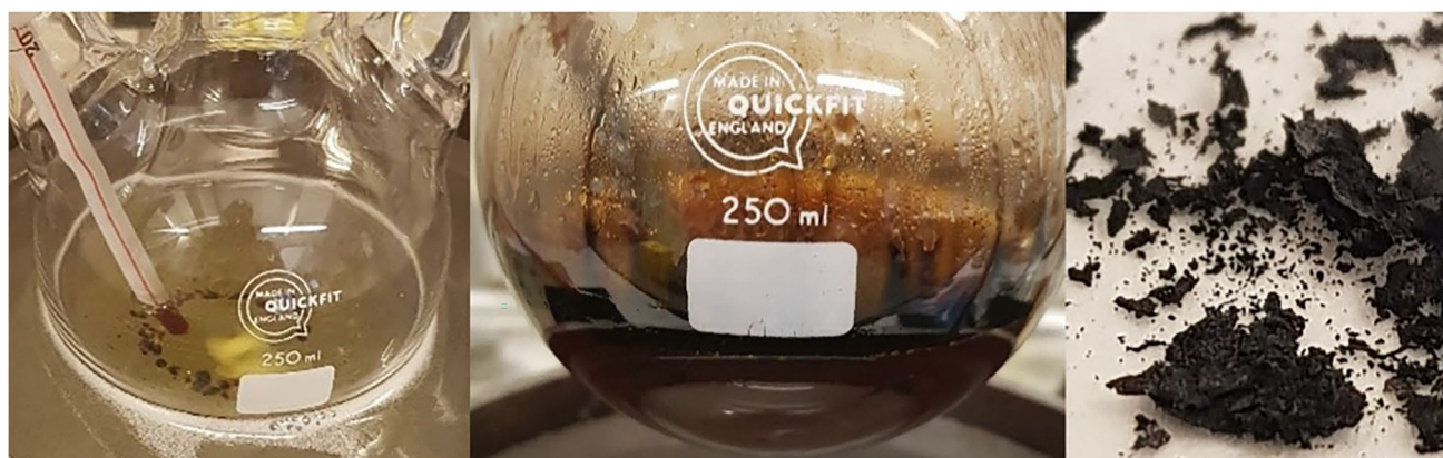
Fig. 9 Pictures showing the formation of black particles in laboratory experiments (experiment 6.1). Separate droplets of furfural collecting on the bottom (L). Black liquid and particle formation (M) dried particle residue retrieved from the flask (R)
