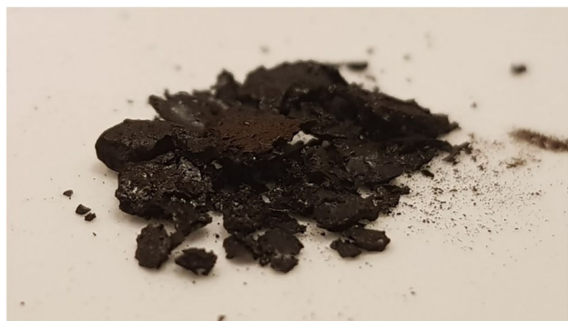
Fig. 4 Picture of a sample of black particles found in the distillation unit (sample #5, Table 1)
