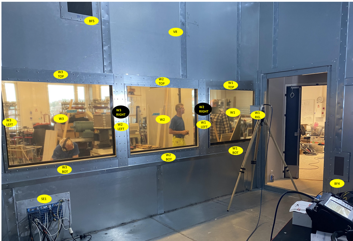
Figure C.7: Location of test points on north wall of shielded enclosure. Photo: Daniel Asle Vingen Endal.
