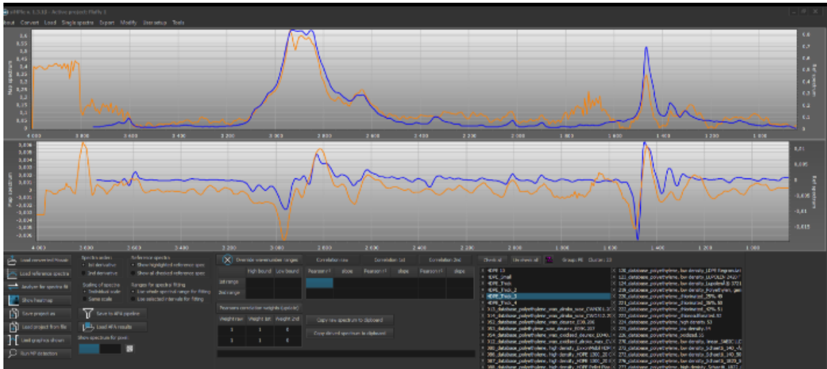
Figure 88B- Comparison spectra using SiMPle reference library with PE polymers found in the sample (orange) to the standard (blue).
