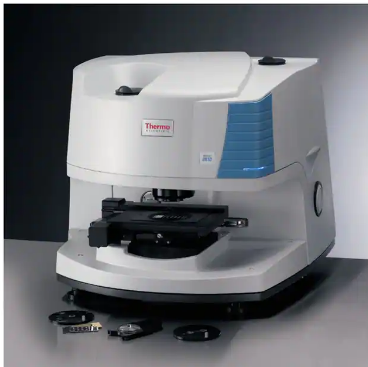
Figure 17- Model of the Nicolet™ iN™10 MX Infrared Microscope used in this study (Thermo Fisher 2022).
