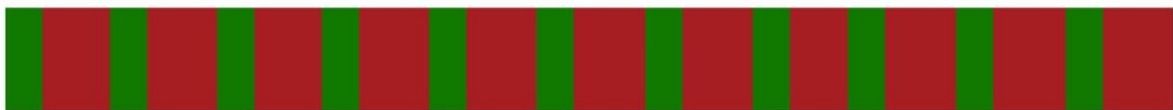
Figure 7.7 Schematic of the Base surfactant-alternating-gas (SAG) injection strategy. The green periods represent surfactant injection and the red periods represents CO 2 injection.
