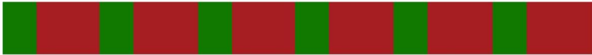
Figure 7.9 Schematic of the Extended surfactant-alternating-gas (SAG) injection strategy. The green periods represent surfactant injection and the red periods represents CO 2 injection.
