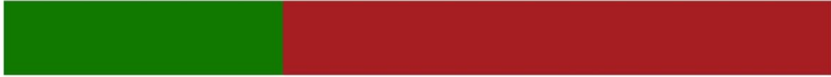
Figure 7.8 Schematic of Single Cycle surfactant-alternating-gas (SAG) injection strategy. The green period represents surfactant injection and the red period represents CO 2 injection.
