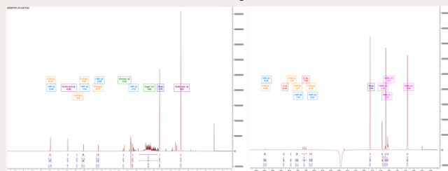
Figure 5: qNMR result after stage 1 (left) and after stage 2 (right) showing that all the sugar/carbohydrates (green) are converted in stage 2.
