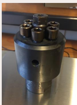
Figure 6: Closed 25mL Parr reactor used in stage 3
