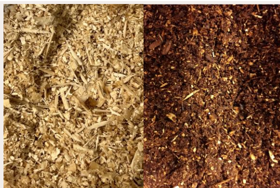
Figure 1: Wood shavings before (left) and after (right) steam-explosion. The steam-exploded shavings (right) are used as feedstock in this project.
