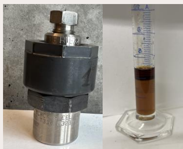
Figure 3: Left: Closed 20mL Parr reactor used in stage 2. Right: Phase separation of the aqueous and organic phase after reaction.
