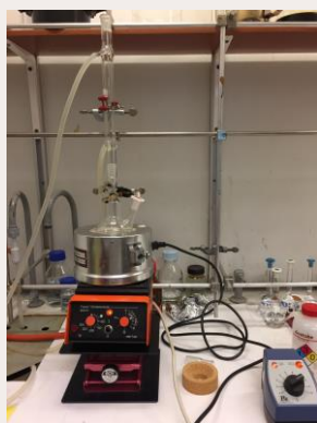
Figure 2: The setup of the acid hydrolysis
