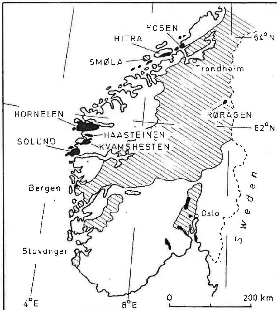
Fig. 2.2. Locations of the main areas of O.R.S. sediments in Norway (black). The ruled area represents the approximate extent of the Caledonian nappes and autochthon. The remaining white areas are Precambrian crystalline basement (after Roberts, 1983).
