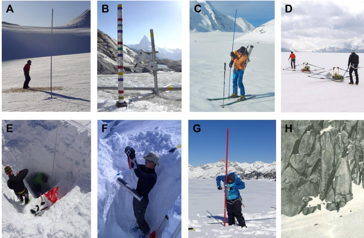
Figure 2.4 Field measurement of mass balance: (A) Stake for snow depth measurement (B) automated stake (C) snow probing, (D) snow thickness measurement with ground-penetrating radar, (E) snow pit excavation (F) snow density measurement, (G) snow coring for snow density measurement, (H) markers painted rocks to monitor snow surface changes (Nivometer)). Geibel et al, 2022; Photos: M. Huss (A, E-G), C. Ogier (B-D), P. L. Mercanton (H).
