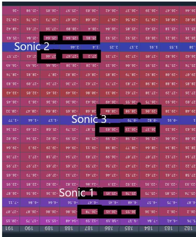
Figure 4.3: CNR - array in the area surrounding the SA positions. The position of the SAs is estimated in the center of the 6 black boxes.
