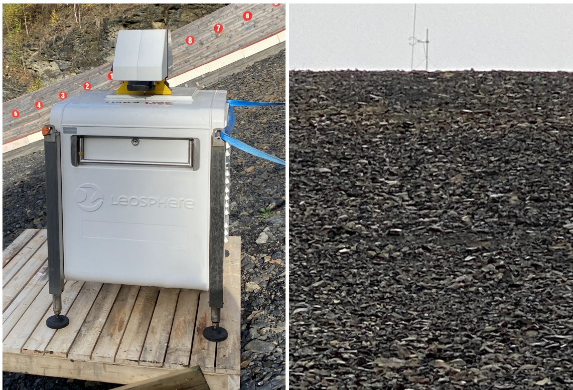
Figure 3.5: left: Scanning LiDAR of type WindCube 100s from Leosphere (WC100s) in its operating position in the slope of the ski jump hill. right: Sonic anemometer S3 seen from the position of the WC100s. Note that the scan plane hits at the S3 sensor height in the default PPI scan
