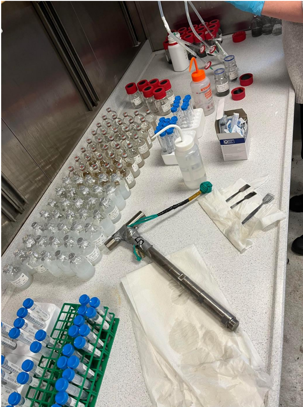
Figure 5: Image of one of the titanium incubators and subsampling after retrieval.
