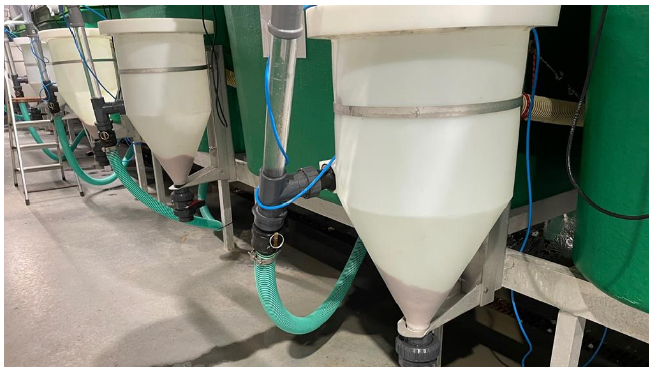
Image 1: Experimental tanks installed with feed collection system used in the study. Image Credit: Ernst Hevrøy.
