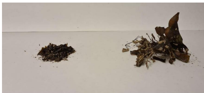
Figure 6: Freeze-dried epiphyte biomass. Left: processed by cutting, chopping, and grinding. Right: unprocessed freeze-dried material.
