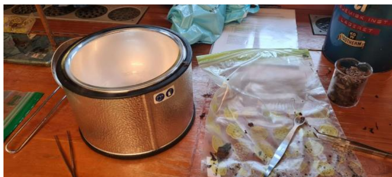
Figure 8: Equipment used for liquid nitrogen drying algal epiphytes, including liquid nitrogen Dewar flask and processed epiphyte biomass in a beaker.
