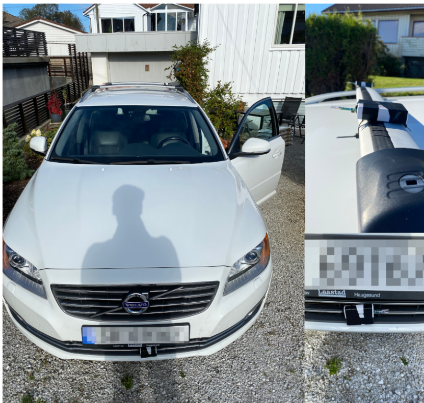
Figure 2.5: Instrument mounts used at the proof of concept trial and roof mount for main runs for the Haugesund route, left: car overview, top right: roof mount, bottom right: iMet mounted on bottom
