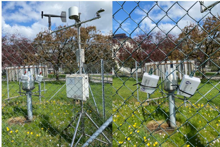
Figure 2.2: Garden instrument setup in front of the GFI, iMets on the fence, and reference instrument on the mast behind, this is an example, with the same setup as the benchmark, but fewer iMets
